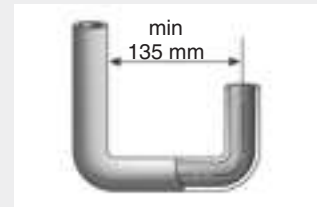
● Minimum clearance of U-shape bends
