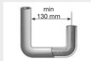
● Minimum clearance of U-shape bends
