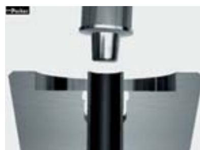
After starting the process, the dies clamp the tube and the flanging pin starts the orbital movement and the forward stroke
