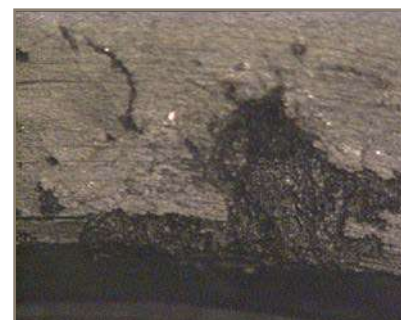
Pitting on filter end-cap
